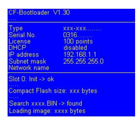
The display shows different information such as the network settings, the serial number and the number of license points. If the Flash card does not contain an operating system, the screen shows the following:
